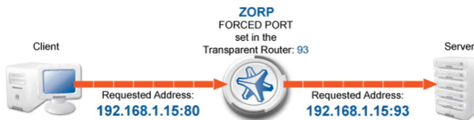
Figure 6.31. Using TransparentRouter with the Modify target port option
